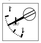
This gage shows the engine coolant temperature.
